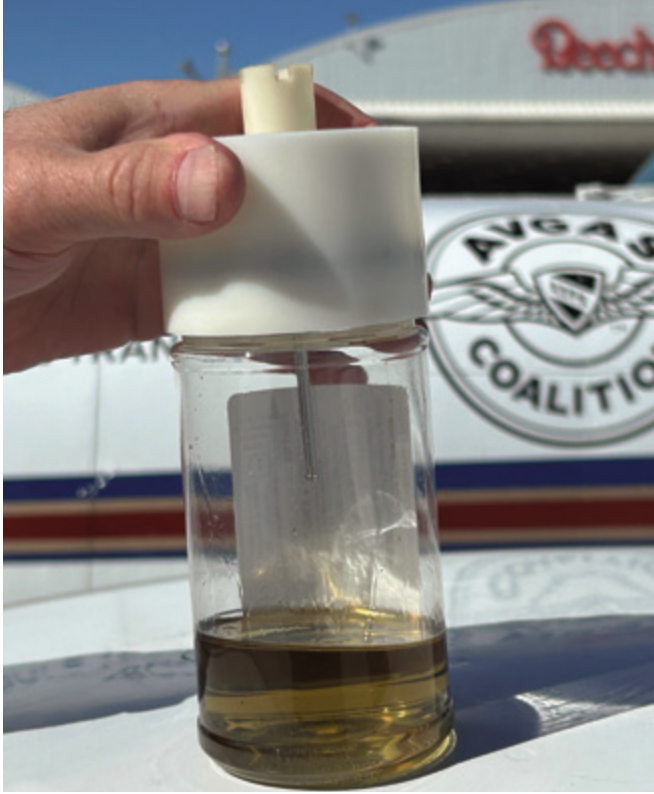
Photo 4: G100UL's "native" color is dark yellow. When commercially available blue dye will be added to make the fuel green, distinguishing it from jet fuel.
