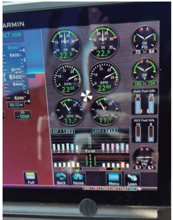
Photo 7: Matched fuel flow. G100UL on the left, 100LL on the right
