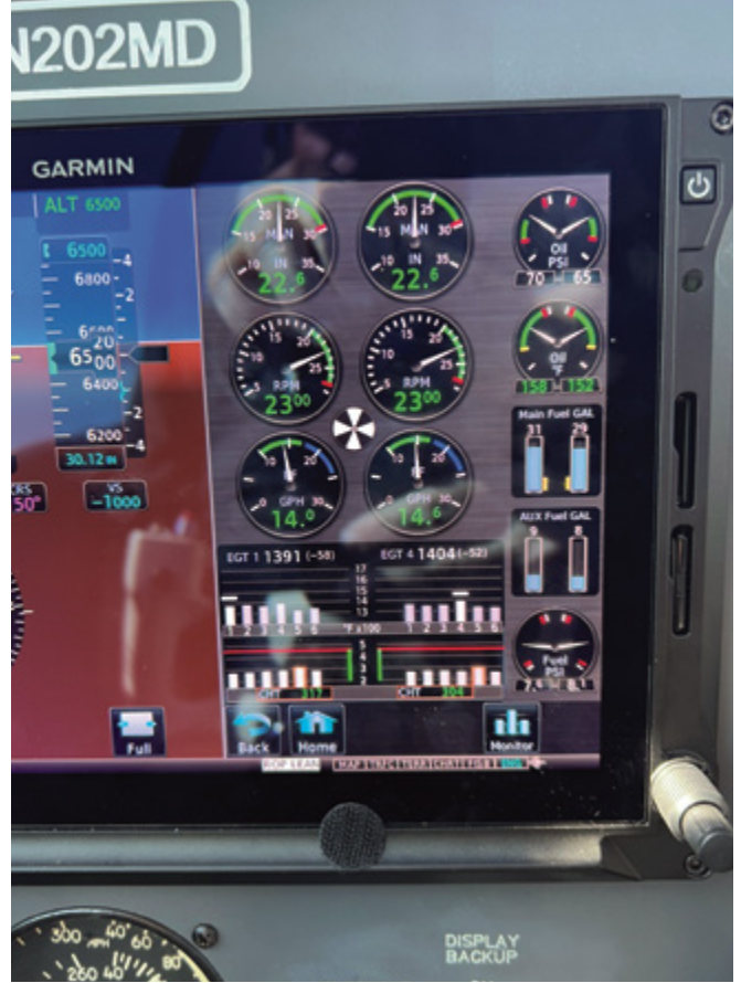
Photo 5: Engine data at about 50°F rich of peak. G100UL on the left engine, 100LL on the right
