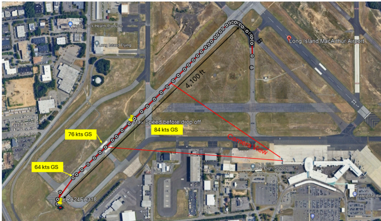
Figure 1 - Preliminary ADS-B data with the airplane's track over runway 24 overlaid along with annotations of the airplane's ground speed.
