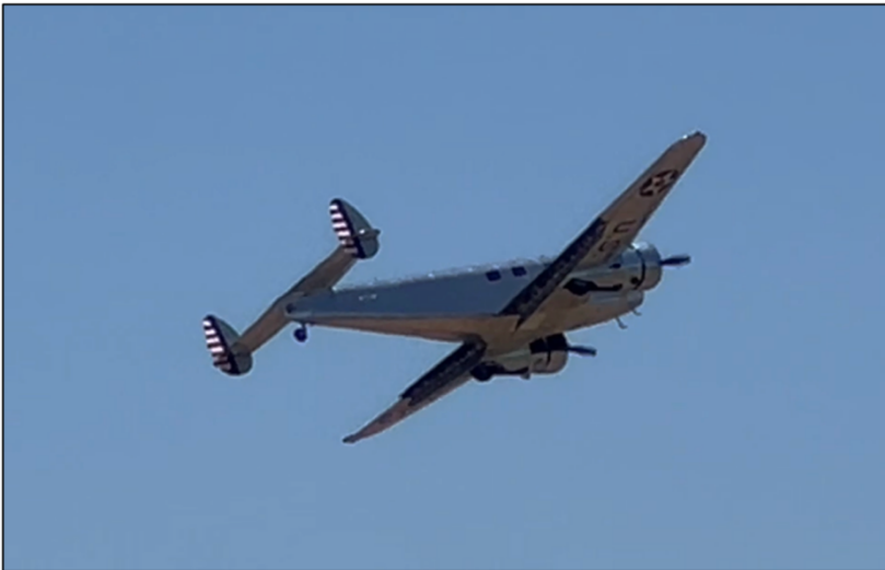
Figure 1: Screen capture of witness provided video of the accident airplane with the flaps extended during the takeoff climb.
