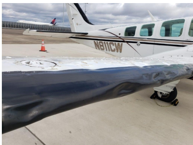
Figure 1. Leading edge damage to right wing (provided by FAA)
