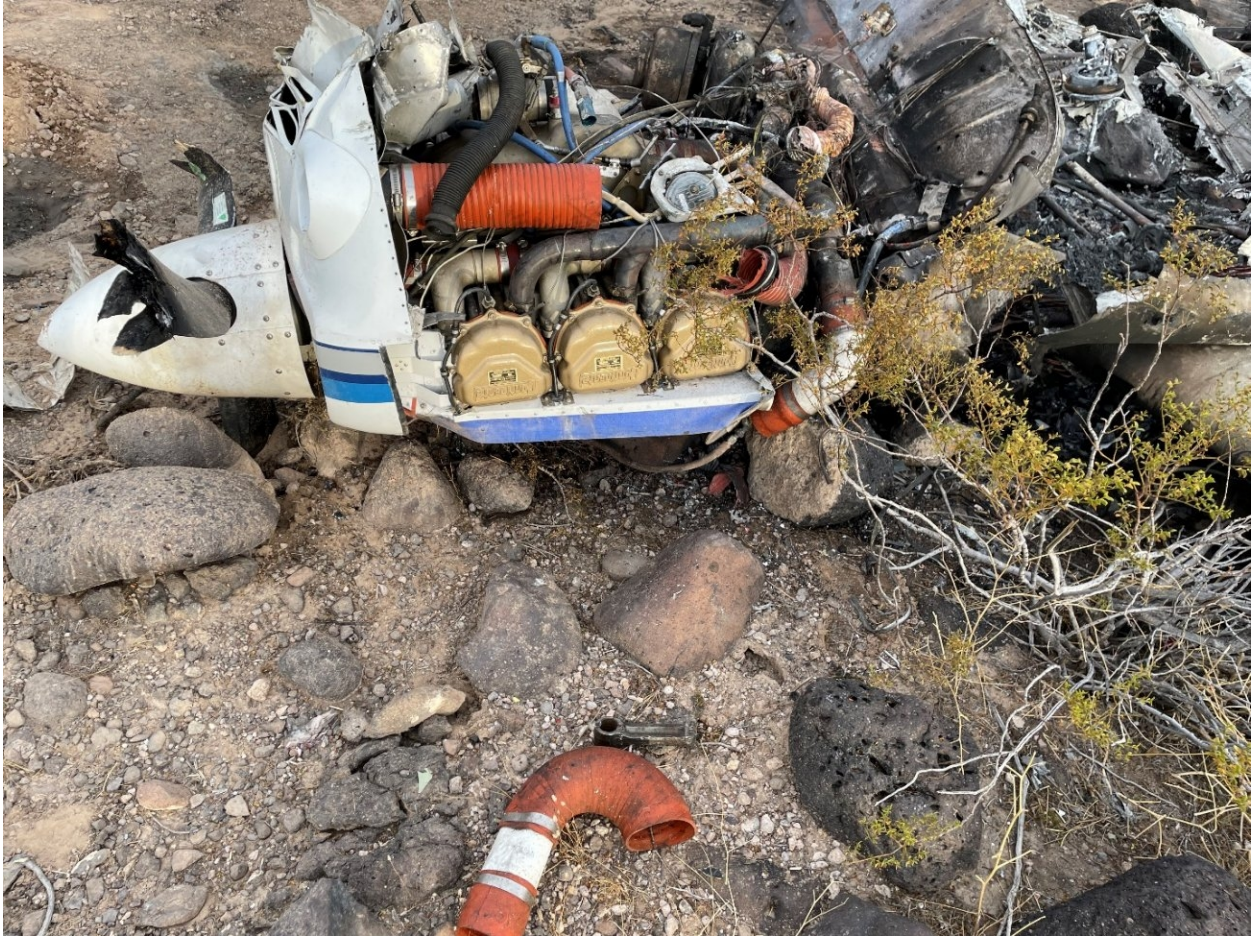
Figure 1: Post-accident image of connecting rod on the ground next to engine (Courtesy of LEA)
